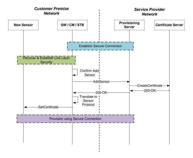
Figure 1 – Automated Certificate Installation Sequence Diagram
