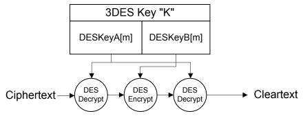
Figure B.3-3 - 2-key Triple DES, EDE-121 mode, Decryption
