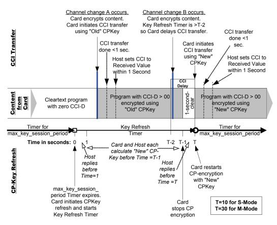
Figure 9.4-2 - Two Examples of CCI Transfer During CPKey Refresh
