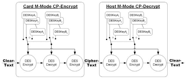
Figure 7–3 - M-Mode Encryption
