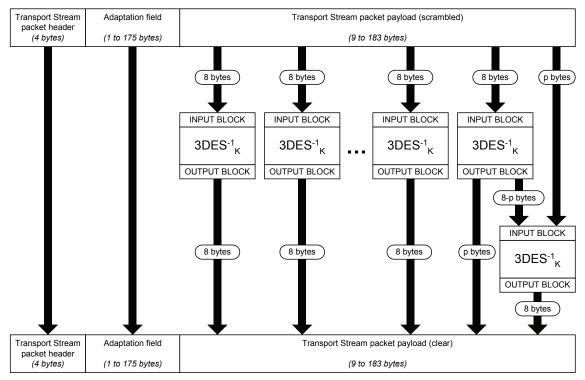
Figure B.3-7 - MPEG Transport Packet Descrambling, Case 2
