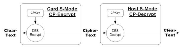
Figure 7–2 - S-Mode Encryption
