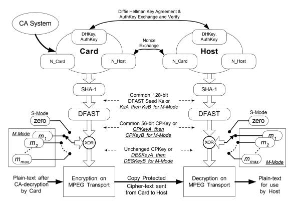
Figure 7–1 - Encryption Key Generation
