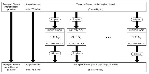
Figure B.3-4 - MPEG Transport Packet Scrambling, Case 1
