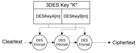
Figure B.3-2 - 2-key Triple DES, EDE-121 mode, Encryption
