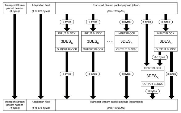
Figure B.3-6 - MPEG Transport Packet Scrambling, Case 2
