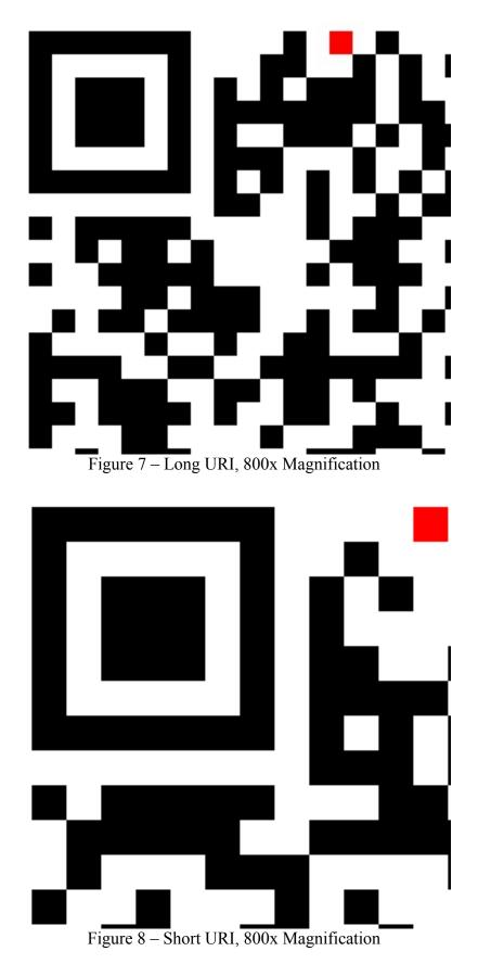
In Figure 7, the minimum size of a "module" (shown by the red dot) is 16x16 pixels. In Figure 8, the minimum size of a "module" is 24x24 pixels. The larger size of the "module" generally results in increased readability of the code from a further distance.
