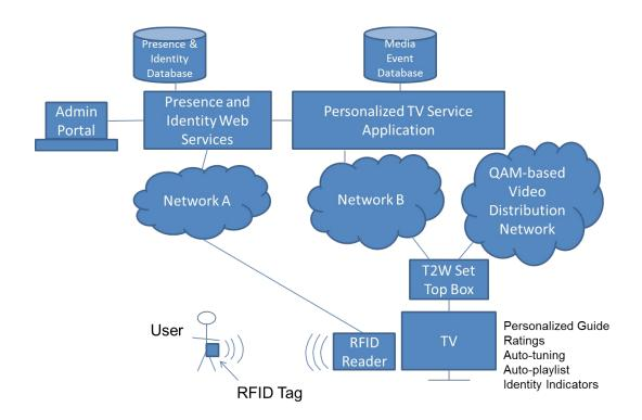
Figure 1: High-Level Diagram of the use of an RFID tag and RFID reader to detect user presence and identity and report to a personalized television service application
