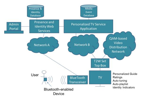
The figure below demonstrates how the same process can be implemented with Bluetooth rather than RFID.
